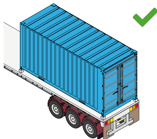
Figure 232 Loaded container with doors to the rear
