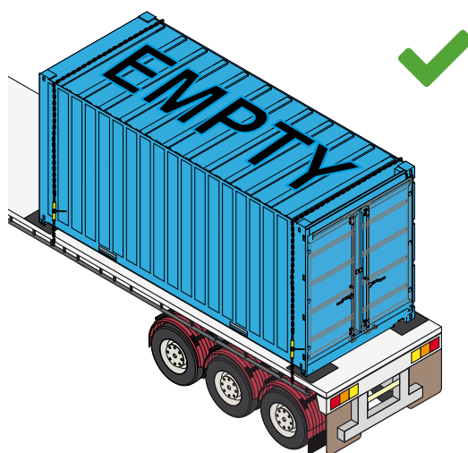
Figure 230 Empty container cross-chained
