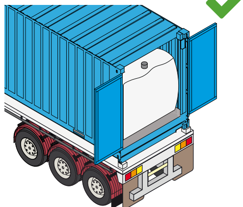
Figure 238 Flexible tank product surge
